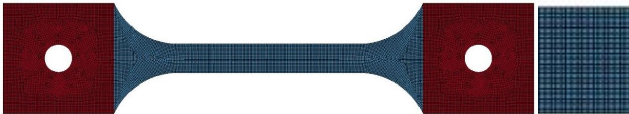
Figure 11. Mesh 5 – 20 Elements through the Cross Section with a Close-Up View
