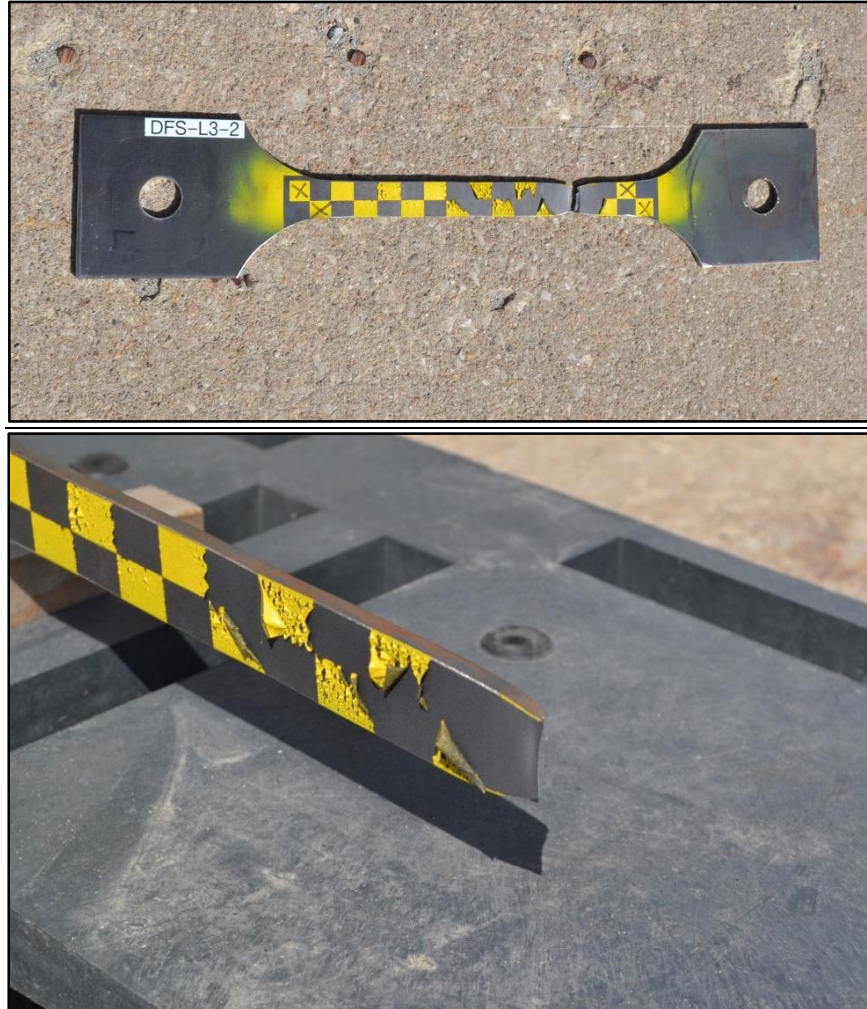
Figure 44. Post-Impact Photographs, Test No. DFS-L3-2
