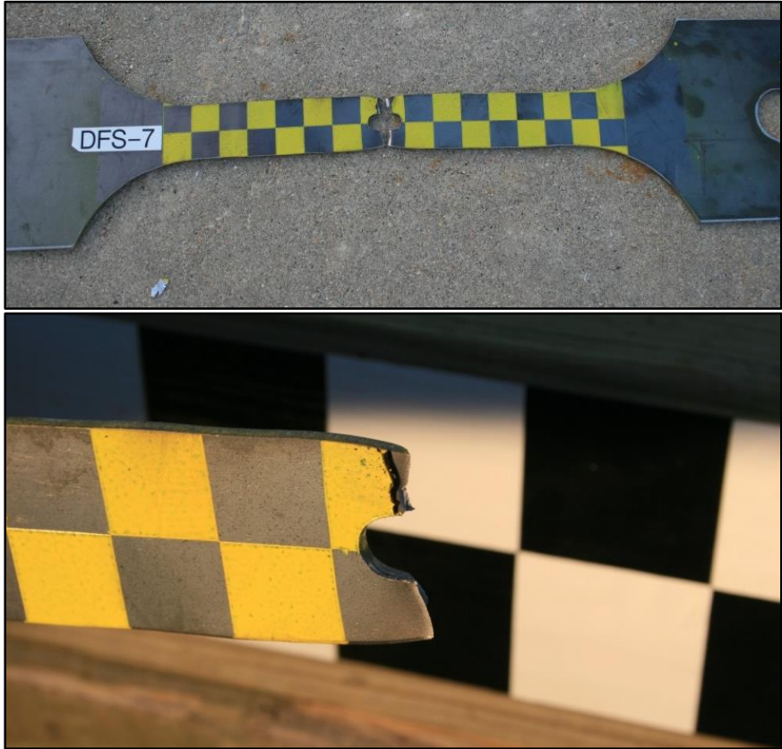
Figure 56. Post-Impact Photographs, Test No. DFS-L7
